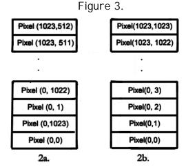
Image data as transferred directly to system memory from a Dalsa CA-D4 twochannel camera and 2b after hardware reordering into scan line order by a frame grabber.
